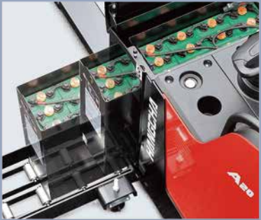
Side battery change is standard feature
